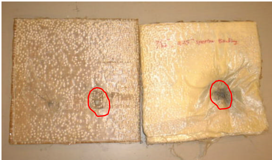
Figure 2.7: Damaged Areas on the Facing and Backing Layers of Panel After Ballistic Impact
